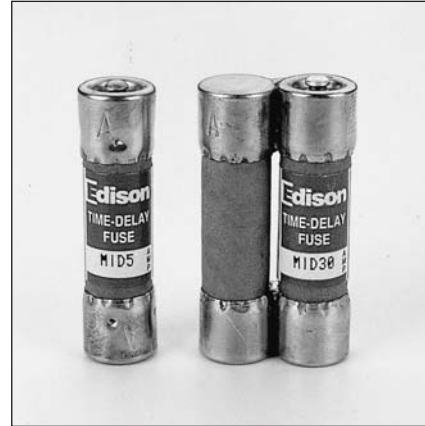
Catalog No. MID (.1 - 30A) .1 - .8A 250 Volts AC or Less 1 - 15A 125 Volts AC or Less 20 - 30A 32 Volts AC or Less Pin Indicating - Time-Delay
