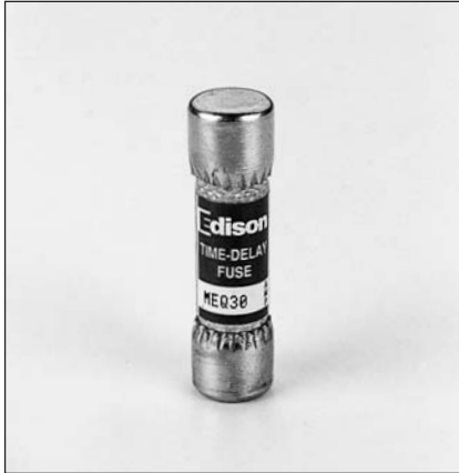
Catalog No. MEQ (.1 - 30A) 500 Volts AC or Less Time-Delay
