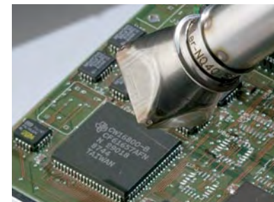
Patented Weller nozzle technology safely removes QFPs, PGAs, and SMT bases.
