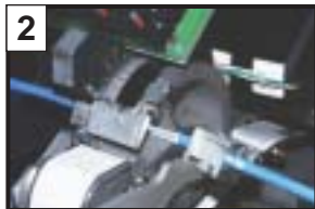
2 Pressing the foot pedal begins wrapping the label on the cable
